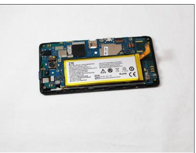
• Use a plastic opening tool to lift the press-fit connector up and disconnect the battery ribbon cable.
