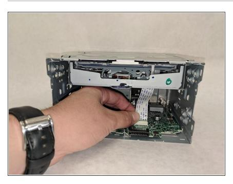
Remove the ribbon wire from where it is being held in place. This can be done by applying force upwards.
