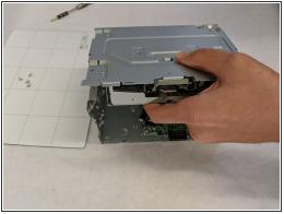
Unscrew the four 7.3 mm outer screws on the top to remove the top face from the rest of the frame.
