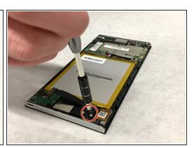
Using the T-5 bit, unscrew the three 5mm screws, two attached to the green board, one attached to the black board.
