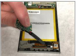
Using the nylon spudger, remove the silver cylindrical component followed by the green then black components
