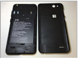
Pry open the back cover from the crease at the bottom left corner with opening tool or fingernail.
