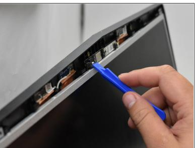
Use the plastic opening tool to disconnect the screen from the top mount.
