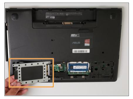
Slide the hard drive to left and remove it from the device.
