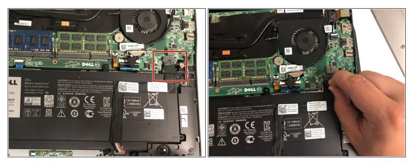
Disconnect the battery from the motherboard by pulling the black tab attached to the cable.
