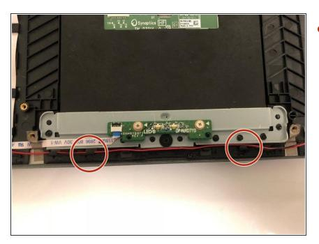
Untangle the wire from the plastic clips and remove the speakers from the device.
