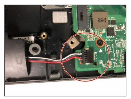
Remove the ribbon cable by pulling it out.
