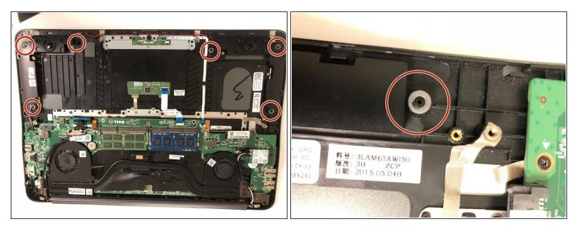
• Remove the compression caps by using the spudger.
