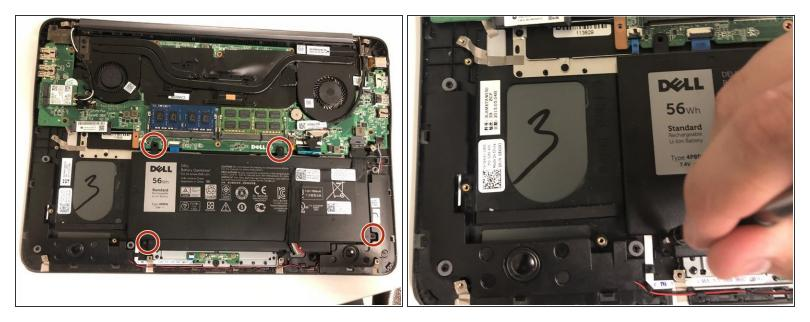
• Remove the four 2.5x6mm screws using a Phillips #1 screwdriver.
