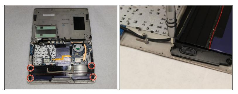
• Unscrew the 4 1mm PH00 screws attaching the speakers to the frame.
