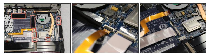
• Remove the motherboard connector cables by gently lifting the black latch that clamps them in place with a spudger or simply pull the connector from the port.
