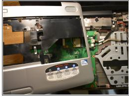
Using the opening tool, carefully go around the edge and loosen the palm-rest assembly, until you can comfortably and easily lift it off.
