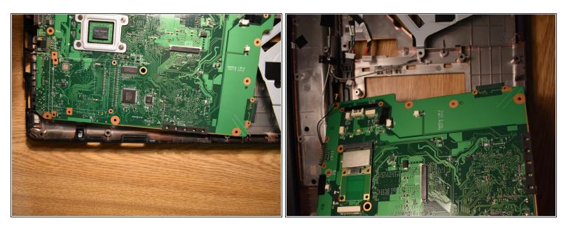
Once ready to remove the motherboard, carefully pry it away from the bottom first, as to not risk damage to the chassis, since the volume wheel sticks out of the motherboard to the exterior.
