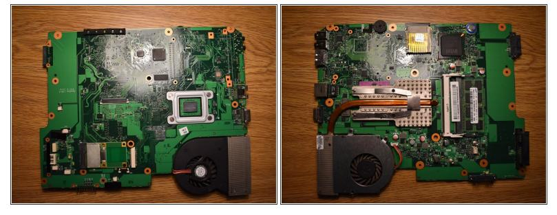
Separate the motherboard from the device and flip it over.
