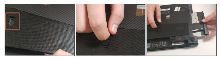
Hold this lock down while removing the optical drive.
