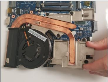
Unscrew the six screws using a Phillips #0 screwdriver.
