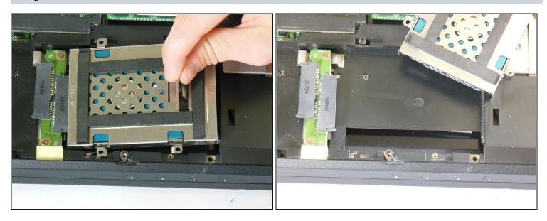
• Remove the hard drive, lifting gently by the tab as shown.
