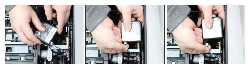
• Remove the adapter by pinching the plastic head of the wire connector and pulling it out of the port.
