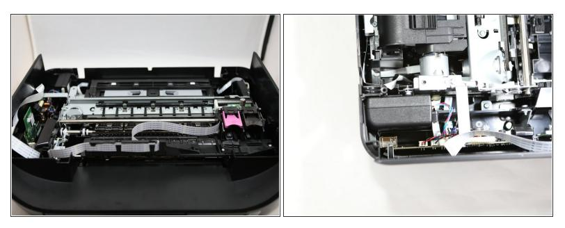
(i) Locate the the AC adapter at the top left corner of the device which is connected by intertwined red and blue wires.
