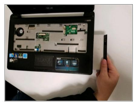
Slide the disk drive out of the device.
