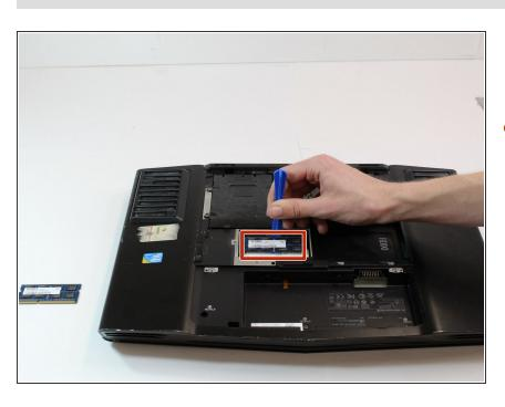
For the second RAM card use the opening tool to gently lift the RAM card forward. To reassemble your device, follow these instructions in reverse order.
