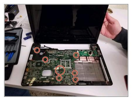
Unscrew and remove the marked screws.
