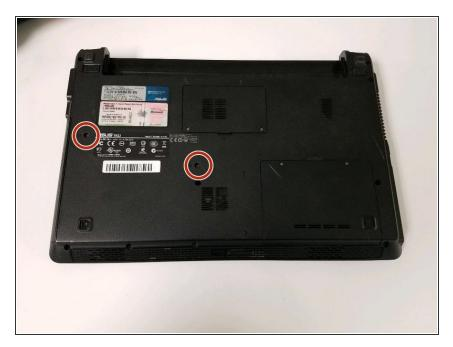
Use the Phillips #0 screwdriver to remove the two screws on the back of the laptop.
