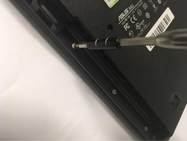
Rotate the laptop until it is sitting face up and extract all screws exposed by removing the keyboard.
