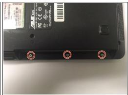
Remove all screws located on the bottom plate of the laptop, beginning with the three located underneath the disc drive.
