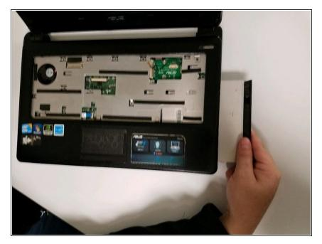
Slide the disk drive out of the device.
