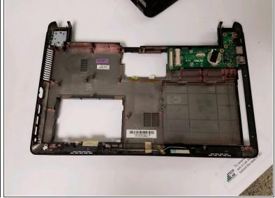
Remove the motherboard from the device.
