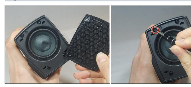
• Remove the 4, PH1, 15mm screws on the side speaker cover frame.
