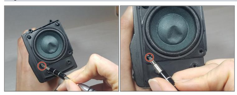
• Remove the 4, PH1, 10 mm screws from the subwoofer frame.
