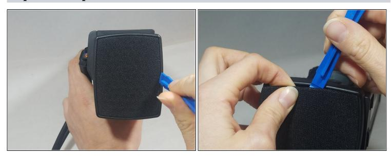
• Using the blue plastic opening tool, pry up on the cloth covered end panel. The edge of end cap cover should separate from main body of device.
