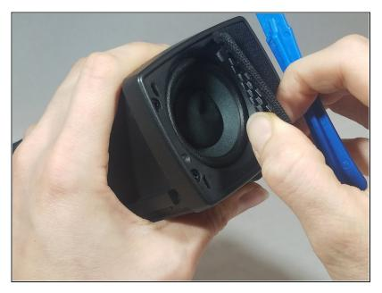
Using your fingers, lift up on the end cap cover until it separates completely from the main body of the device.
