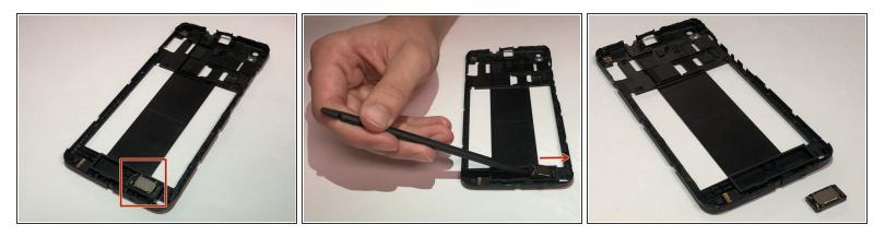
• Use the spudger to pry out the speaker from the Frame Cover.
