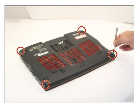
Using the Phillips #0 screwdriver, unscrew each of the four screws on the back of the laptop case. The screws are 0.5 inches long.
