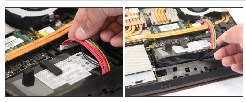
Disconnect the battery cable. Pry the battery out using the black nylon spudger.
