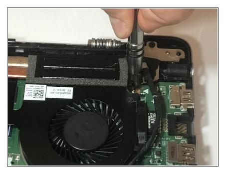
Remove the 6mm PH1 screw from the motherboard.
