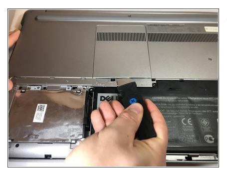
Pry up the plate covering the RAM, using the metal jimmy.
