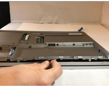
Close the laptop and flip it over exposing the bottom surface. Use the metal jimmy and blue opening tool, gently pry the bottom cover off. Repeat this process around the entire perimeter of the laptop.
