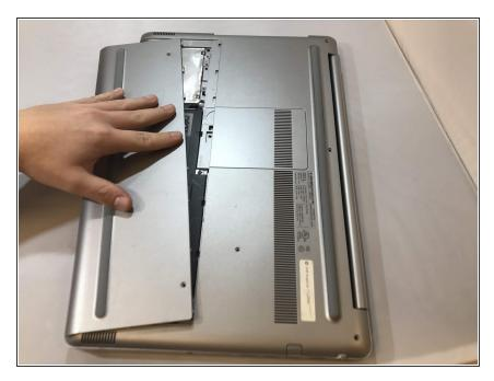
Apply pressure with your fingertips on top of the cover and drag toward the front of the laptop. This will make the plate slide off exposing the hard drive.
