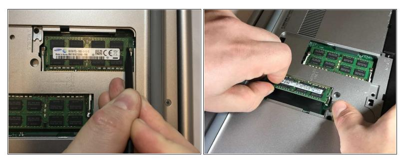
• Apply outward pressure using fingers or a spudger on the small tabs on the RAM. Once freed the RAM will need to be lifted slightly, angling it upward, and then pulled out toward yourself.
