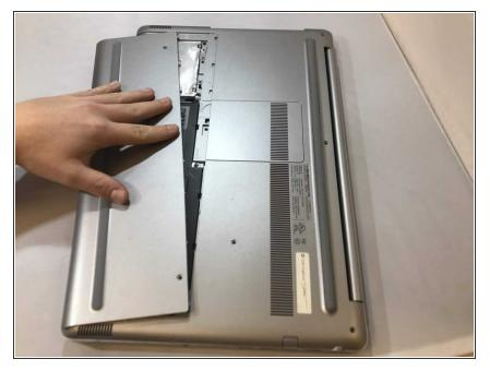
• Apply pressure using your fingertips on the top of the cover and push toward the front of the laptop. This will make the plate slide off exposing the hard drive and battery.
