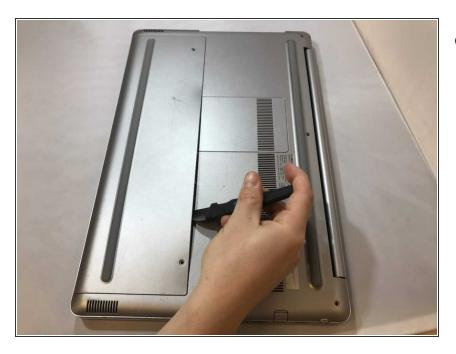
• Using the metal jimmy, pry up to remove the first half of the cover.
