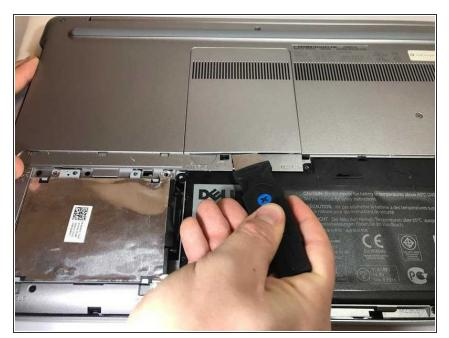
• Using the metal jimmy, remove the cover plate, this will expose the RAM.
