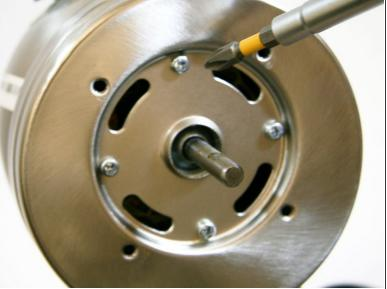
Remove the four 6 mm bolts and small washers that secure the front face of the motor housing with a Phillips #3 screwdriver and remove the washers.
