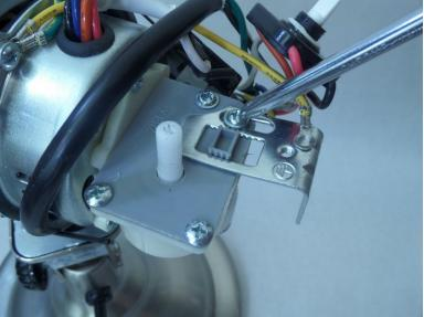
Using a Phillips #3 screwdriver unscrew the 13 mm long screw fastening the motor housing support to the oscillation gear box.
