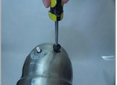
• Unscrew the 10 mm screw in the center hole of the oscillation knob with a Phillips #3 screwdriver.
