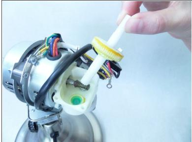
Remove the upper oscillation gear.
