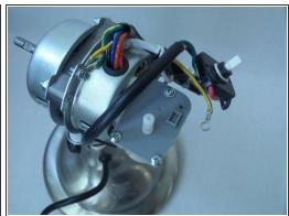
Using a Phillips #3 screwdriver, unscrew and remove the 7 mm long bolt and small washer fastening the yellow and green wire to the motor housing support.
