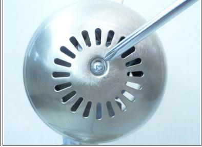
• Remove the 10 mm triangular-headed bolt with a Phillips #3 screwdriver.
