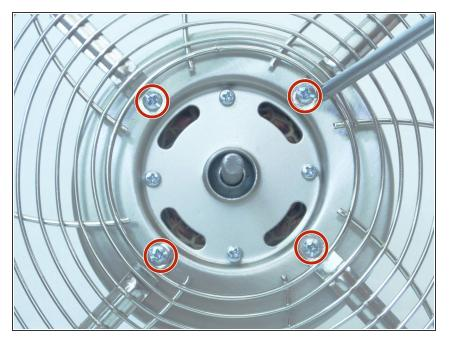
Unscrew the four 8 mm bolts that fasten the back of the fan cage back to the motor housing with a Phillips #3 screwdriver.
