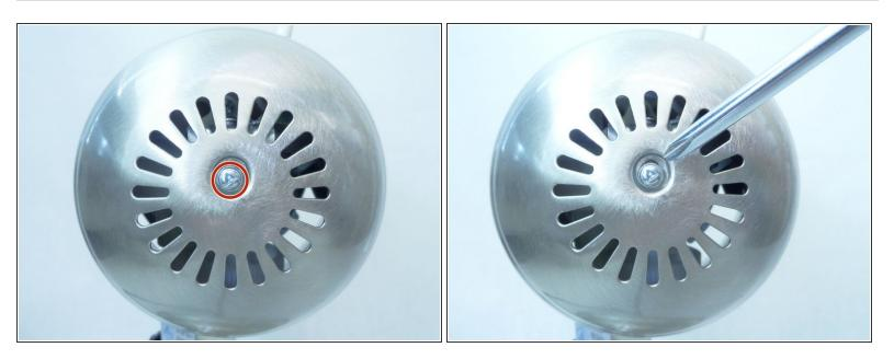
• Remove the 10 mm triangular-headed bolt with a Phillips #3 screwdriver.
