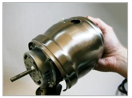
Slide the back end of the motor housing away from the front of the rotor.
