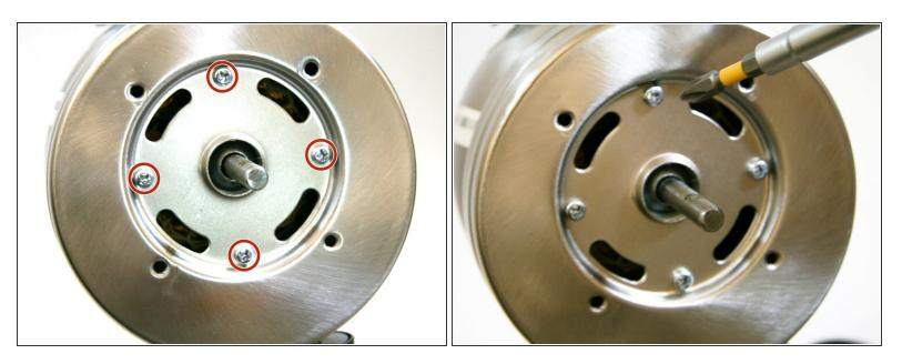
Remove the four 6 mm bolts and small washers that secure the front face of the motor housing with a Phillips #3 screwdriver and remove the washers.
