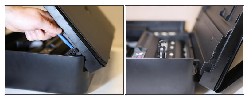
• Remove the clip holding the scanner bed up by using the plastic opening tools. Prying the clip away from the the side of the scanner bed.
