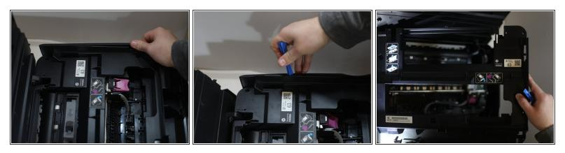
• Using the plastic opening tools, pry between the outer shell and the main plastic frame.
