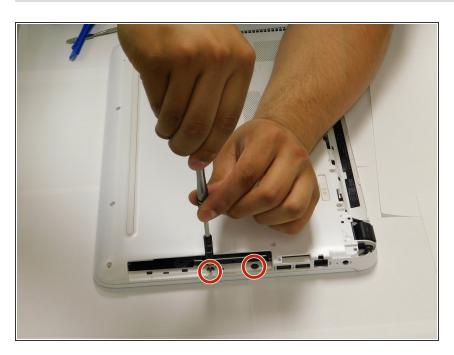
Unscrew the two 3.5mm silver screws with the Phillips #000 and the Philips # 1.
