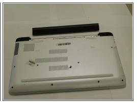
Slide both tab buttons inward to open the battery cover. Gently push the battery out to remove.
