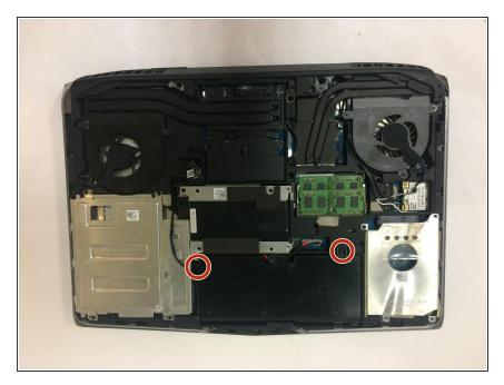
Remove the two 5.5 mm Phillips #0 screws holding the battery in place.
