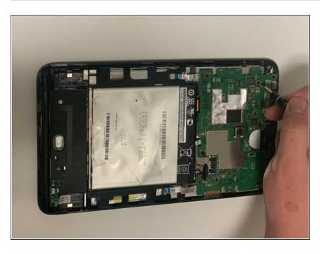
Remove the six screws holding the motherboard in place using a Phillips #000 screwdriver.
