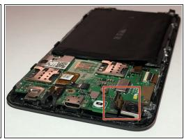
Pry off the low profile connector located on the right side of the camera device.
