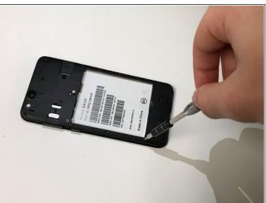
Remove the sixteen 3 mm screws on the back cover of the phone using the Phillips #000 screwdriver.
