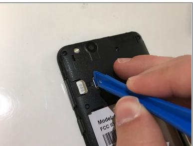
With a spudger, gently push the sim card away from the center of the phone to remove it.
