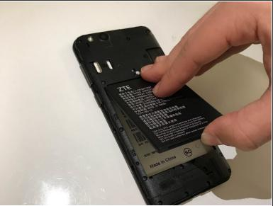
Find the divot near the bottom of the battery and remove the battery from the device.
