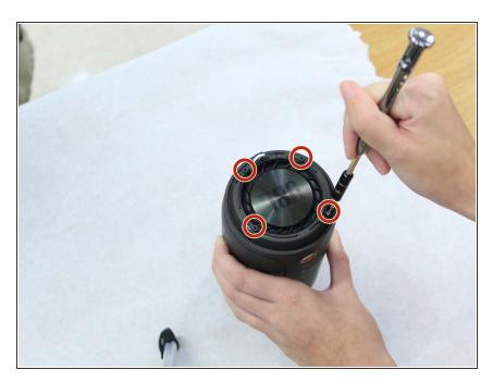
Remove the four 9.5mm Phillips #1 screws from each end of the device.
