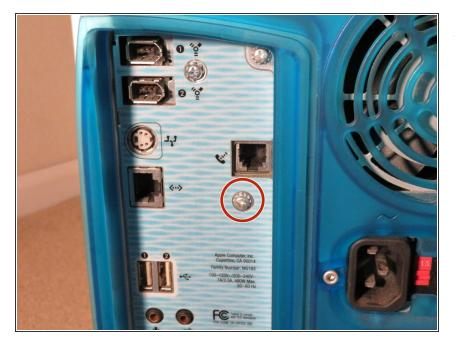
Remove the Phillips #1 screw circled in the picture. Set it aside for reassembly.
