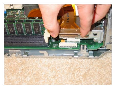
Disconnect the modem's flex cable from the connector on the logic board.
