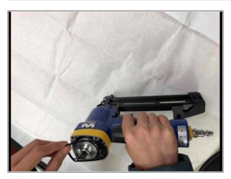
Remove the faulty gasket and replace it with a new gasket.
