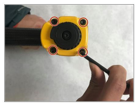
Using a 4mm Allen wrench, remove the 4 Allen screws, 44mm in length, from the yellow cap on the back of the brad nailer.
