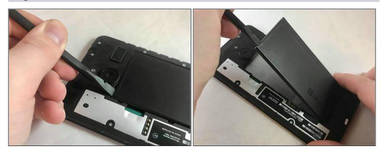
• Lift the battery away from the phone with the flat side of a spudger.
