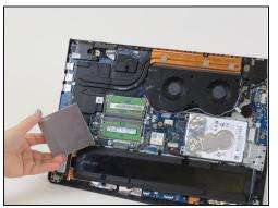
• There will be a silver square box next to the fan. Use a plastic spudger to pry the small tabs on the side that are holding the silver square on.
