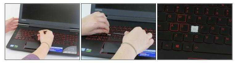
• Carefully remove the broken key(s). Use the flat end of the spudger to gently pop the key off.
