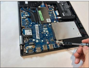
• Remove the three 4 mm screws using a Phillips #00 screwdriver.
