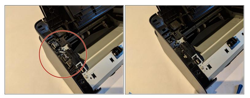
• Once the housing is removed, remove the three buttons.
