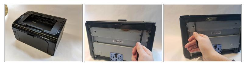
• Flip printer on it's back. Using the plastic spudger, pry off front panel. There will be two main points to focus as shown.
