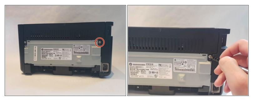
Unscrew the #1 Phillips screw 6mm on the back of the printer.
