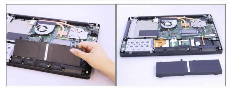
• Once the screws have been removed, gently lift the battery out.
