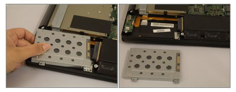
• Gently disconnect the Hard Drive from the connector cable. Lift it out and remove it.
