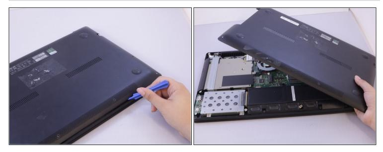
• Use an opening tool to pry open the rear cover. Lift the cover off and away from the board.
