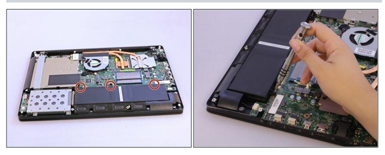
• Use a Phillips #0 screwdriver head to remove the three black 7mm Phillips head screws that hold the battery in place.
