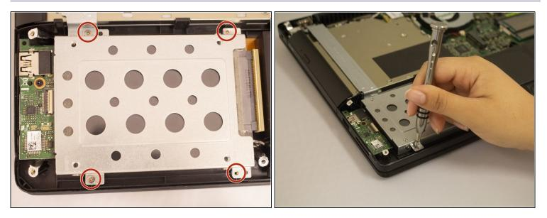
• Use the Phillips #0 Screwdriver to unscrew the four silver 5mm screws.
