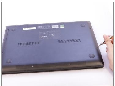
Use a T4 Torx screwdriver head to remove the ten 4mm Torx head screws on the bottom of the laptop.
