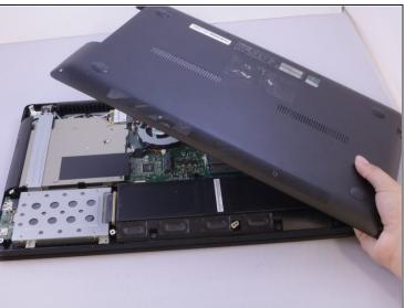
• Use an opening tool to pry open the rear cover. Lift the cover off and away from the board.
