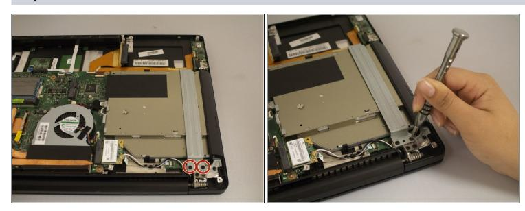
Use the Phillips #0 screwdriver to remove the two 7mm Phillips head screws from the metal disc drive holder.
