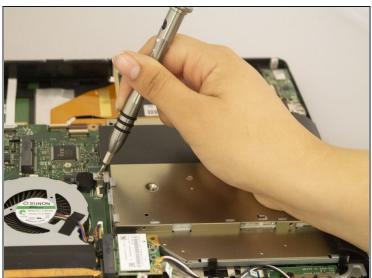
• Use the Phillips #0 screwdriver to unscrew the one silver 5mm Phillips head screw that connects the disc drive to the motherboard.
