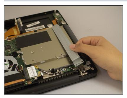
Lift the metal disc drive holder off of the disc drive to remove it.
