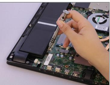
Use a Phillips #0 screwdriver head to remove the three black 7mm Phillips head screws that hold the battery in place.
