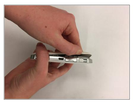
Using your finger, pry open any of the four corners of the back case of your AirCard 770S, until you see the back case disconnect from the device.
