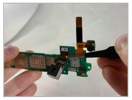
• Disconnect the rear facing camera from the motherboard with tweezers.
