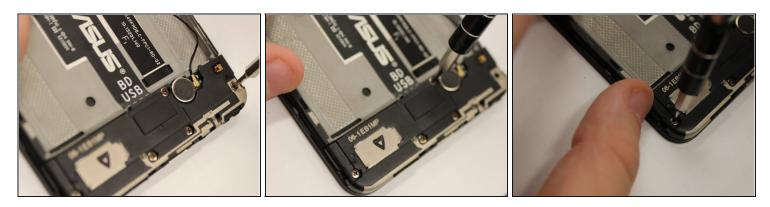
• Remove all screws 3mm, using the Phillips #00 screwdriver, at the bottom of the device.
