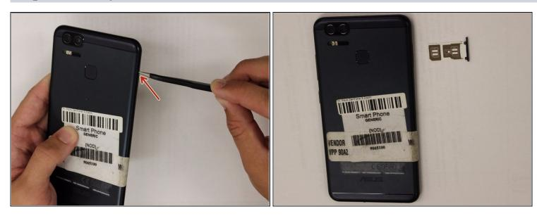
Using a pair of tweezers, pull put the SIM card tray and set it to the side.
