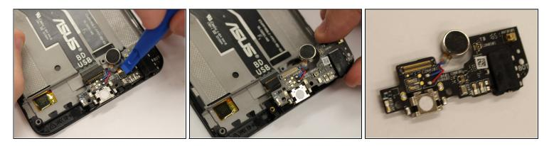
• Using the pry tool, pry up the circular piece and remove the board.
