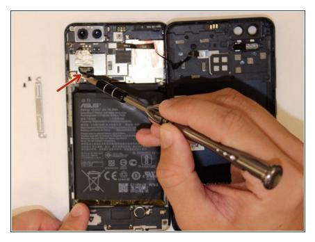
Disconnect the battery connections.
