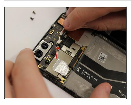
Unplug the wire connecting the two large pieces of the device. Next, seperate the two halves of the phone.
