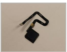
• Using the plastic opening tool, pry the fingerprint scanner out.
