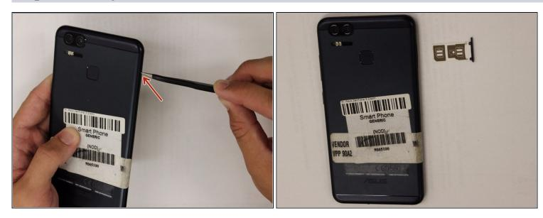
• Using a pair of <u>tweezers</u>, pull put the SIM card tray and set it to the side.
