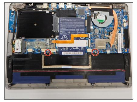
With the Phillips #0 screwdriver, remove the two 5 mm screws that are located above the long black piece of the battery.
