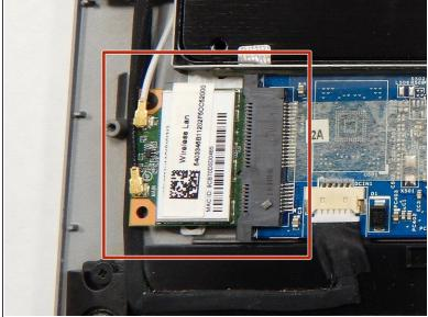
• Locate the Wi-Fi card (it is near the black rectangular hard drive).
