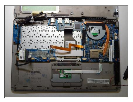
Without bending it, lift the entire battery (both the long black piece and the rectangular blue piece) straight up. Place it off to one side.
