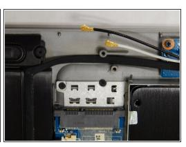
Lift and remove the Wi-Fi card.
