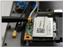
Lift up and remove the two cables attached to the Wi-Fi card (one is white and one is black) with the spudger tool.
