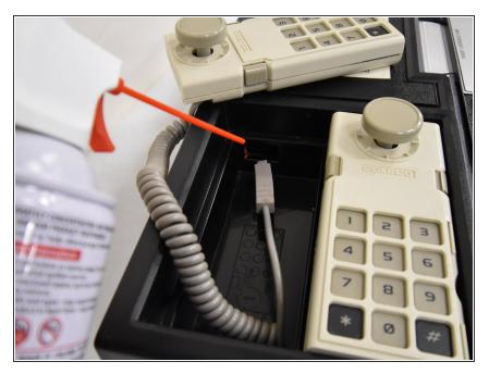
• Spray the insides of the ports a few times with compressed air.
