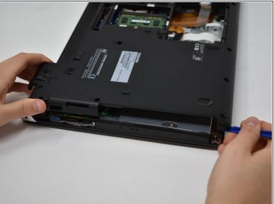
• Insert the plastic opening tool into the edge of the laptop and pry off the back cover.
