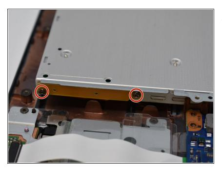
Remove two 2.5 mm screws from the side of the optical drive using a Phillips #0 screwdriver.
