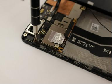
Remove the 3 mm circuit board screws, using the Phillips #00 screwdriver.
