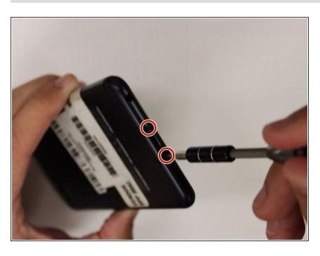
Remove the two 2 mm screws using a Torx T2 screwdriver.
