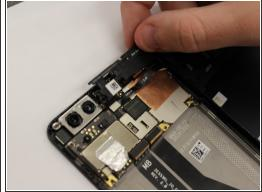
Remove the 3 mm screws, using the Phillips #00 screwdriver, from the black plastic piece at the top on the right side.
