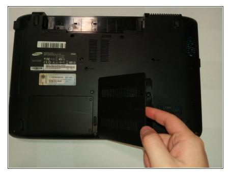
Place the flat end of the spudger or your fingers, if possible, between the panel and the laptop. Pry the panel by moving the spudger up and down until the panel can be removed.
