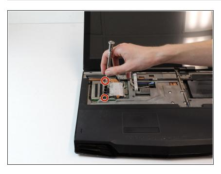
Remove the two 4mm Phillips #1 screws that secure the Graphics Card.
