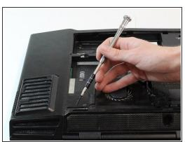
Remove the two 2mm Phillips #0 screws from the recesses on the left and right side of the processor fan.
